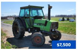
**1979 Deutz-Fahr DX90 Tractor,** Deutz 4.7L 5-cyl diesel 90 hp air-cooled engine, fully synchronized trans., 15 forward and 5 reverse gears, dry disc clutch, up to 25 mph, 4x2 2WD, 7720 lb rear lift capacity, independent rear PTO with wet disc, rear RPM 540/1000, 3-point hitch, standard cab with 2 seats, A/C, front 10.00-16 tires, rear 18.4x34 tires.
