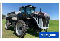
**2020 GVM T325 Prowler,** Cummins 6.7L Stage V 325 hp diesel engine, Funk DF250 4x4 powershift 11-speed auto. trans., 114 in. Dromos fixed axles rated @ 36,000 lb., 2WS, reverse pitch fan, 409 SS painted GVM Double Duty 11-ton spreader body, roll tarp, Raven Viper 4 with RS-1 ISO receiver, Modem and Service Unlock, A/C, AM/FM/BT radio, air ride seat, front fenders, 380/90R46 Trelleborg tires. Warranty options available.
