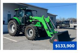
**2020 Deutz-Fahr 6140TTV Tractor,** FARMotion® 4-cylinder 120 hp engine, TTV continuously variable trans., up to 32 mph, 4WD front axle, 32 gpm closed center hydraulics, 4 rear remote valves with flow control, electronic rear hitch control, hydraulic trailer brakes, 15,400 lb rear lift capacity, linkage and PTO controls on rear fender, 3-point hitch, deluxe cab with a high-visibility roof, air ride seat, heat and A/C, sound system, front 480/65R28 R1 tires, rear 600/65R38 tires.
