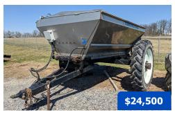
**2012 GVM 8.0T Transpread,** 304 SS, 8-ton capacity, 3-speed gearbox, ground driven, dual spinners, electronic spinner RPM gauge, Shur-Lok roll tarp, 380/90R46 tires. Includes set of 650/75R32 floater tires. Perfect for lime, fertilizer, and cover crop application.
