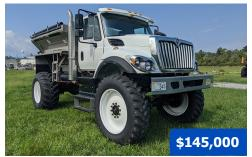
**2019 International 7300 Spreader,** 5000 miles, Cummins B6.7 250 HP engine, Allison trans., 4WD, 409 SS 8 ton GVM Double Duty spreader, Shur-Lok Roll Tarp, Viper 4+ with guidance software, RGL600 light bar, A/C, AM/FM radio with Weather Band, Front Axle, (2) 385/65R34 Goodyear tires, (2) rear 600/60-30.5 floater tires.
